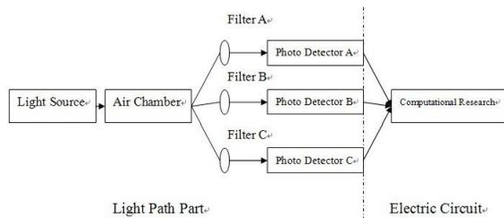
Figure 3. Block diagram of three-wavelength single light path
