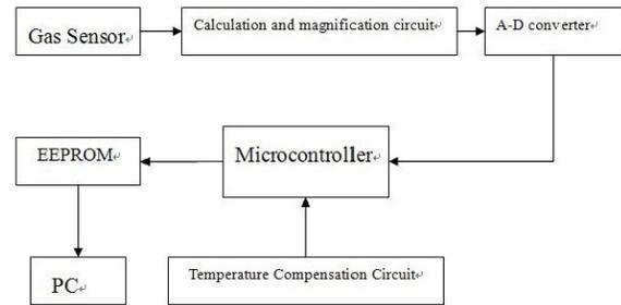
Figure 4. Gas Detection circuit Working Principle Block Diagram
