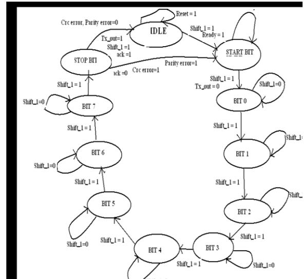
Fig.2 State diagram of receiver
