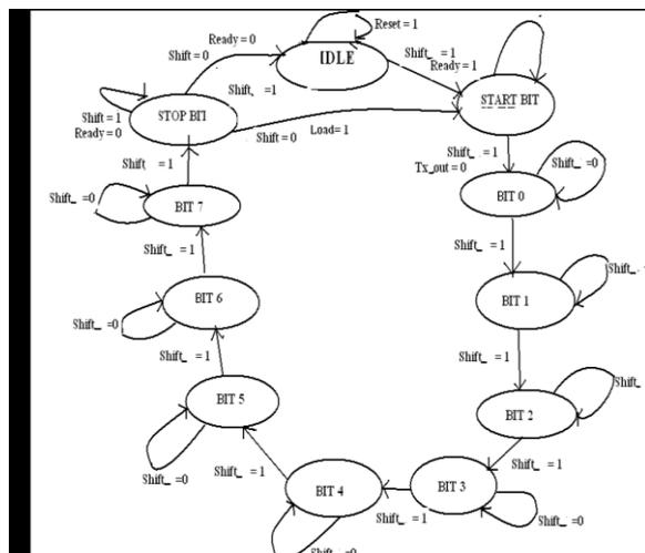
Fig.1 State diagram of transmitter
