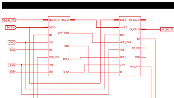
Fig.4 RTL Schematic of UART
