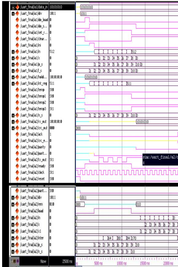
Fig.3 Simulation results of UART
