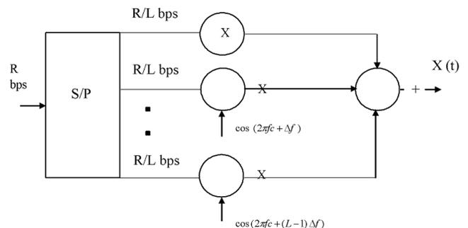
Fig 4. Serial to parallel conversion
