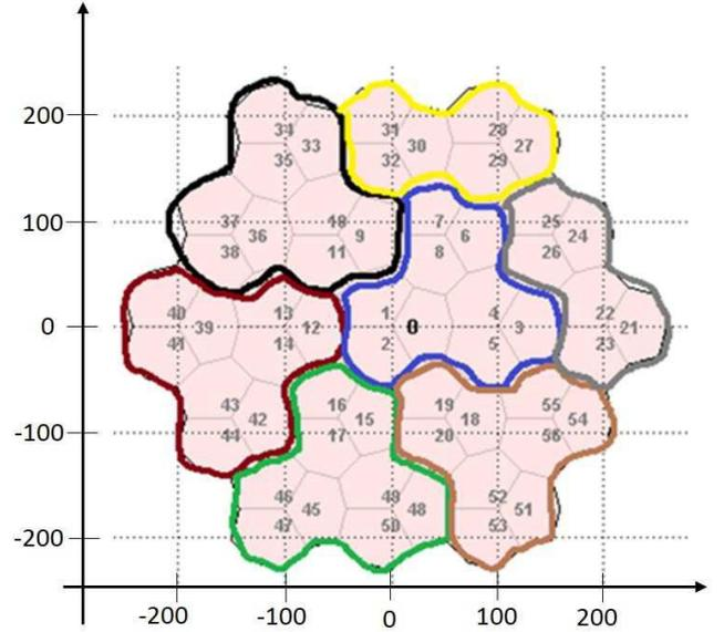
Fig. 2. Pilot-coordination clusters in a 57-cell mobile broadband network. The unit of distance is meters.
