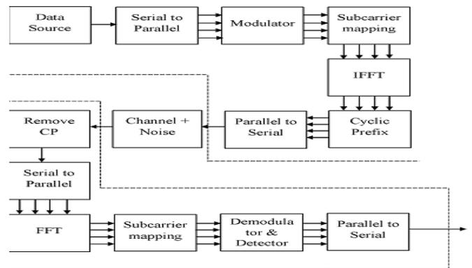
Fig3. Block diagram representation of the OFDM transceiver
