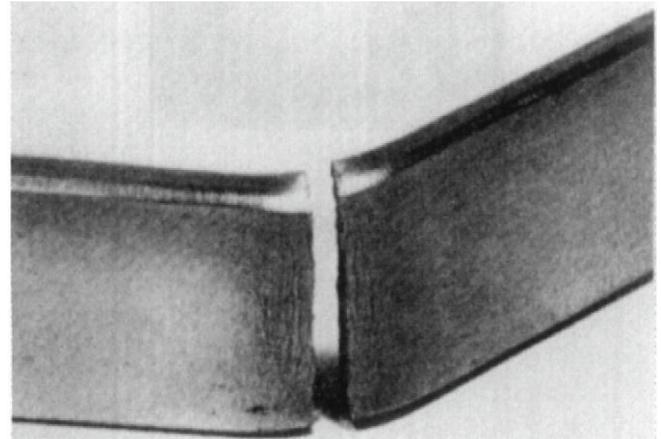
Fig 6: Steel sample after cathodic treatment (x 1).
