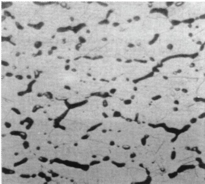
**Fig 2:** Structure of commercial copper after heating in hydrogen for 3 hours at 750°C (about 250 X).
