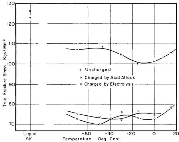
**Fig 2:** Fracture stress as a function of hydrogen absorption and temperature for 0.08% carbon steel.
