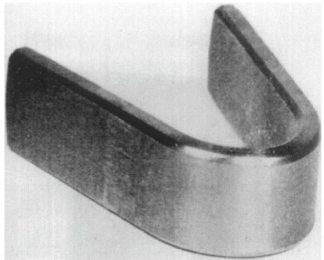
**Fig 5:** Steel sample with no cathodic treatment (x 1).
