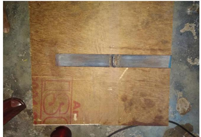
Fig 1: Welded Heat treatable steel plates.
