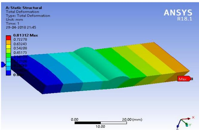
Fig.11 Total deformation
