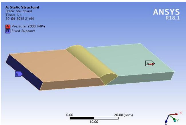
Fig.10 Loads and Constraints
