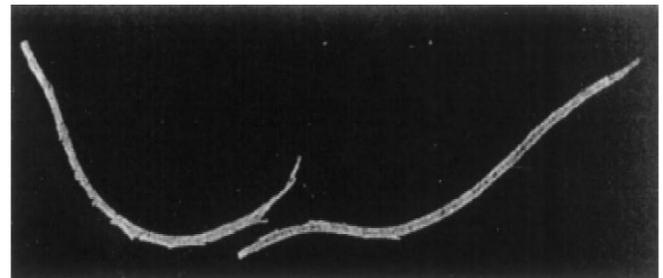
**Fig 4** Vanadium wire shattered by cathodic charging with hydrogen.
