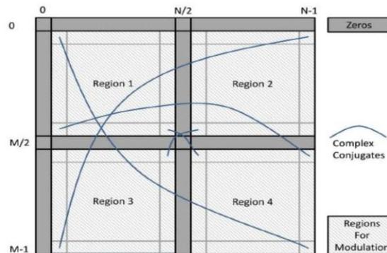
Fig4. Hermitian symmetric matrix used for DPSK-OFDM modulation.
