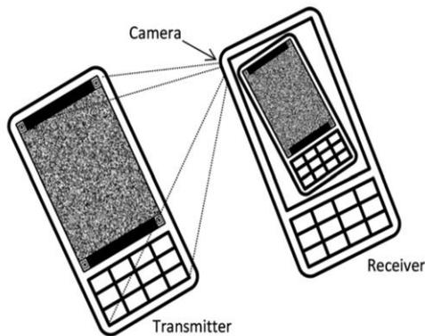
Fig1. transmission of data between two handheld cameraphones using of 2D barcodes
