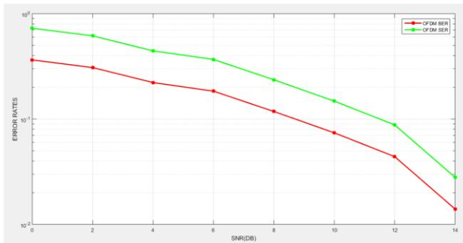
Fig 6. Effect of low pass filtering on BER performance.
