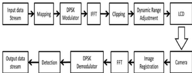
FIG 3. Transmission of information using DPSK Algorithm
